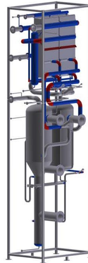
Typical Heavy Hydrocarbon Removal Cold Box 2 MTPA Length – 7.3 m Width – 10.5 m Height – 28 m Weight – 399 t
